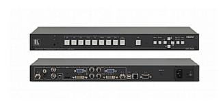
The VP-790 is a high-quality presentation scaler/switcher for RGB component, computer graphics, composite, s-Video, HDMI, DVI and 3G HD-SDI signals. The unit takes one of the inputs, scales the video, embeds the audio and outputs the signal to the computer graphics, DVI/HDMI and 3G HD-SDI outputs simultaneously.
