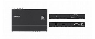
The Kramer VP-427A is a receiver/scaler for HDBaseT twisted pair, HDMI, bidirectional RS-232 and IR signals. The unit receives an HDBaseT signal that it converts to HDMI, IR and RS-232 signals. It up- or down-scales the picture to match the resolution of the HDMI monitor. It includes a simultaneous analog audio output of the embedded HDMI audio.
