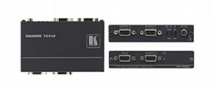
The VP-300K is a distribution amplifier for computer graphics signals with resolutions up to and exceeding UXGA. The unit takes one input, provides correct buffering and isolation, and distributes the signal to three identical outputs.
