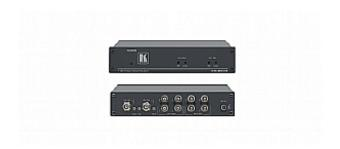
The VM-80VN is a high-performance distribution amplifier for composite or SDI signals. It can also be configured as a 1:4 DA for s-Video (Y/C) signals and has controls to compensate for signal losses inherent in long cable runs.
