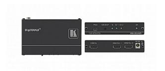
The VM-2UHD is a 1:2 distribution amplifier for 4K@60Hz (4:2:0) HDMI 2.0 signals complying with the HDCP 1.4 content protection standard. The unit takes one HDMI input, equalizes and reclocks the signal and distributes it to two identical outputs.
