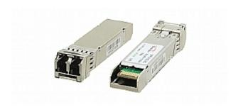
OSP-SM10 is a fiber optic transceiver for 1310nm single-mode signals. This standard pluggable SFP+ module has two LC connectors for reception and transmission signals over two strands of single-mode optical fiber.
