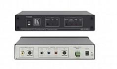
The FC-10Dxl is a high-performance bidirectional transcoder for composite and s-Video (Y/C) signals. The unit converts a composite video or s-Video input through a digital comb filter to a composite and s-Video (Y/C) or component (YUV/RGB) video output.
