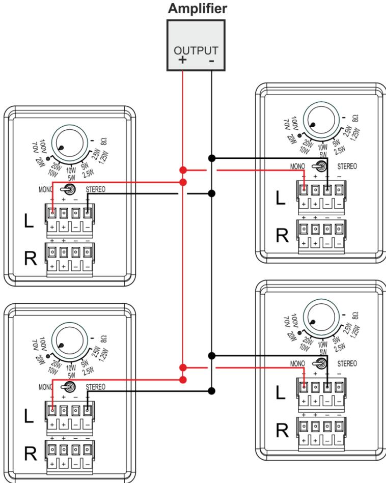
Figure 7: Square Layout Parallel Wiring
