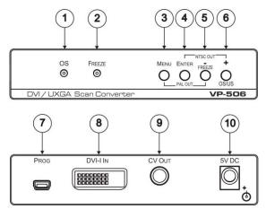
Figure 1: VP-506 DVI/UXGA Scan Converter
