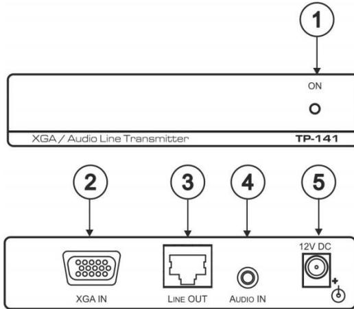
Figure 1: TP-141 XGA/Audio Line Transmitter
