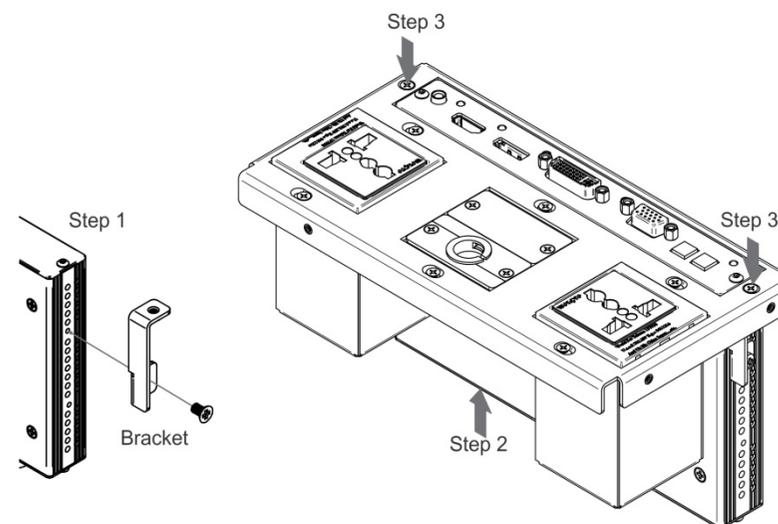
Figure 2: Installing the **SID-X1**
