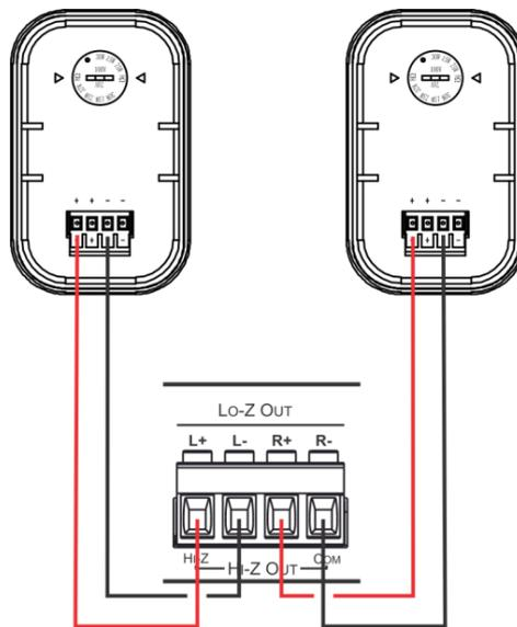
The following diagram displays the **Galil 6-AW** speakers connected to a recommended Kramer power amplifier (for example, **PA-120Z**):
