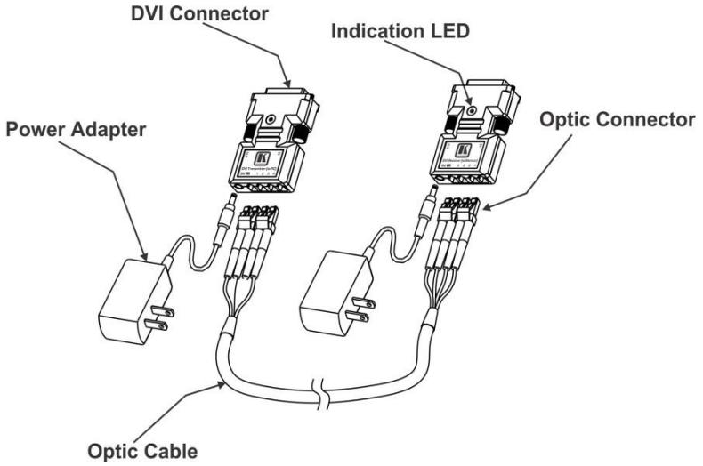
Figure 1: 610 Detachable Optical DVI Transmitter and Receiver
