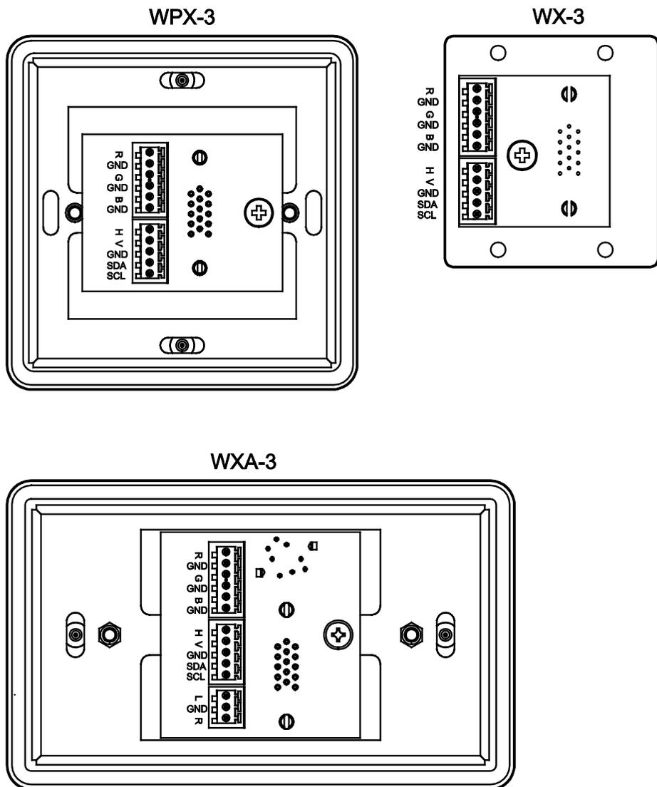
Figure 4: Pinout on Rear Panel
