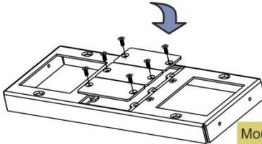
Mount the inner frame into the **TBUS-6xl** enclosure.
