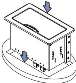
Secure the unit to the table and connect the cables.
