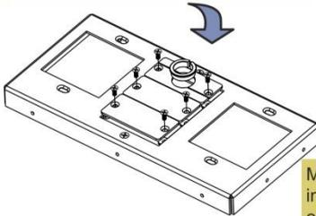
Mount the inner frame into the **TBUS-4xl** enclosure.
