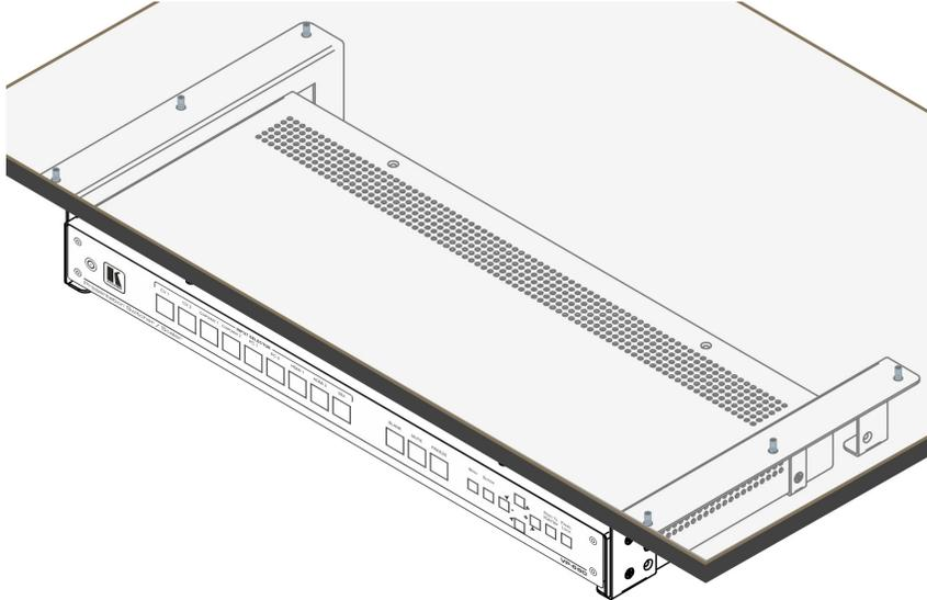
Figure 2: RK-19 Installed under a Table
