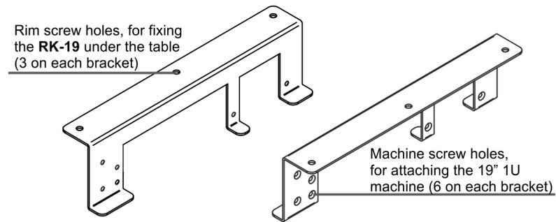
Figure 1: RK-19 Under-the-table Brackets
